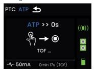
If you get the screen below, it means that the measurement conditions are disrupted. Please check the position of the sensor.
