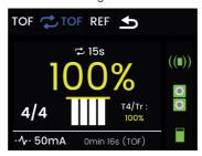
The number of responses detected (TOF count) is displayed as an X/4 ratio (X being the number of muscle response detected).
