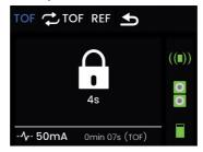
The symbol in front of a result indicates a possible presence of a impaired measurement. The user can do the test again (while respecting the interval) or wait for the next test scheduled in the case of "AUTO TOF" mode.
